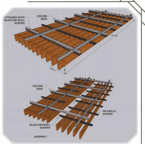
Blade sizes range from 1 3/8" – 4" deep. Our panel width is determined by the project specifications. Solid wood panels are available with 4-10' lengths, and our veneer panels are offered in 8-12' lengths.
