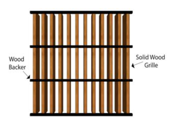
Our panels are nominal 2' wide by 2' or 4' long. Standard blade depth is typically 1-1/2" but can be customized based on the project specifications. The reveal at the panel edge matches the size of the 15/16" T-grid. Optional notched backers can provide more stability for wall installations with blades over 2" deep.
