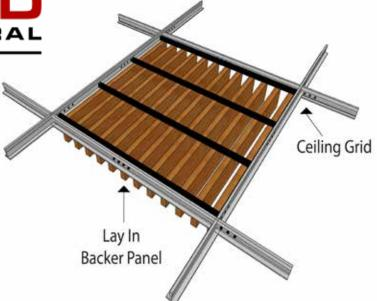
The Lay In Backer panels are factory assembled to "lay into" HD T-grid and typicall require no additiona hardware screws or clips. Solid wood backers are installed on the panels at 12" O.C. and are typically painted flat black - but custom finishes are avaailable per project specifications.
