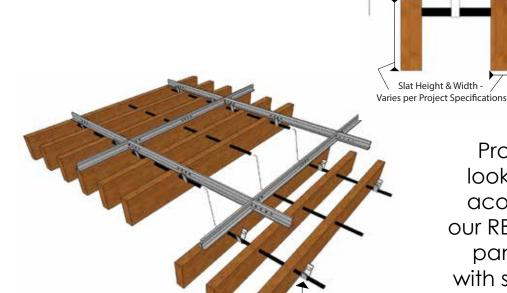
Providing the warm look of wood, plus an acoustical treatment, our RB Dowel Rod Backer panels are available with solid wood or wood veneer options.
