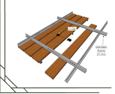
Slats are installed end-toend using our black Linear Open Clips- forming a continuous wood appearance along the space.
